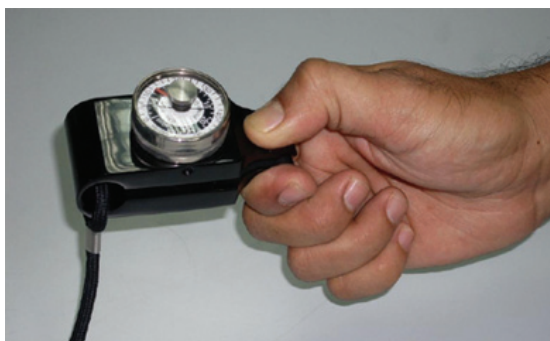
Fig. 2: This figure shows the pinch gauge and how it was used to measure the subject's pinch strength
