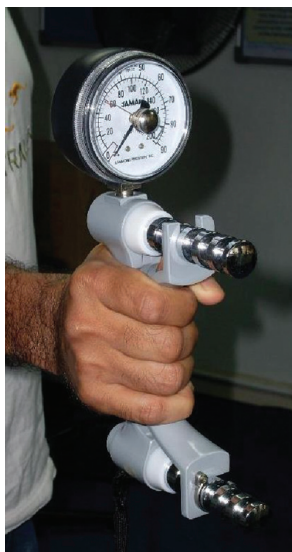
Fig. 1: JAMAR Hydraulic Hand Dynamometer is a standard instrument used in measuring one-handed grip strength
